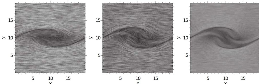
Figure 1: Stream lines in the MHD Kelvin-Helmholtz instability at a Mach number of 0.016 obtained with (left) the HLLD scheme with 256x256 grid resolution, (middle) the new scheme with 256x256 grid resolution, (right) the HLLD scheme with 1024x1024 grid resolution.
