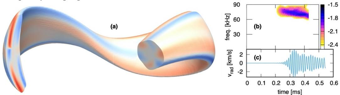
Fig. 1 (a) Radial velocity  $v_{\text{rad}}$  of GAE in three-dimensional form. (b) GAE frequency spectrum. (c) Time evolution of GAE amplitude.
