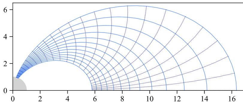
**Fig. 1** A schematic of the flux coordinates at a meridian plane.
