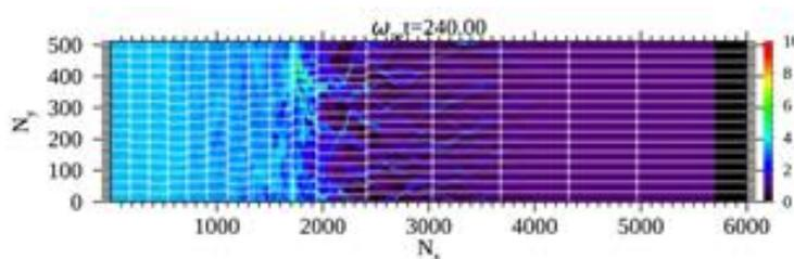
Figure: Relativistic shock simulation by using our new PIC code. Electron density as a 2D color map and the MPI subdomains surrounded by white lines are shown.
