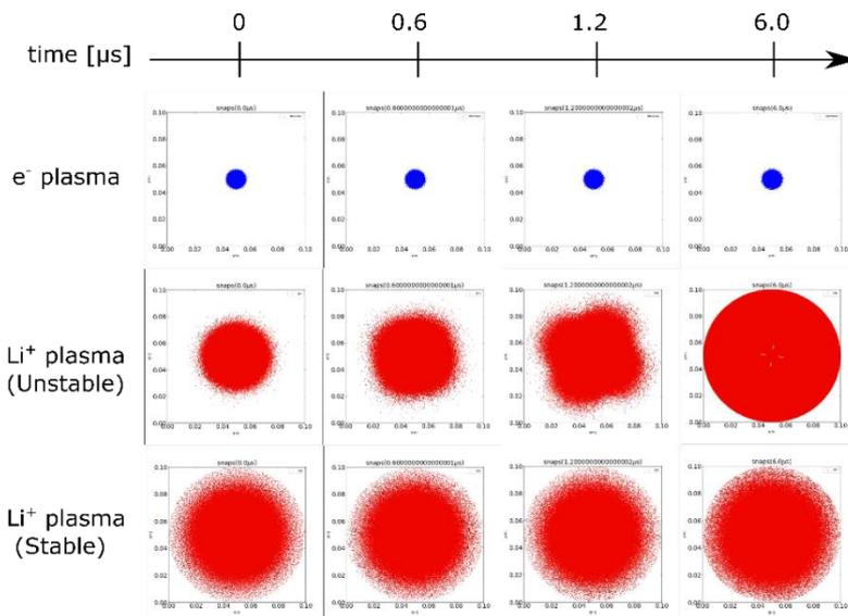
**Figure 1.** 2D profiles of the  $e^-$  plasma and the  $\text{Li}^+$  plasmas for the unstable case and stable one.
