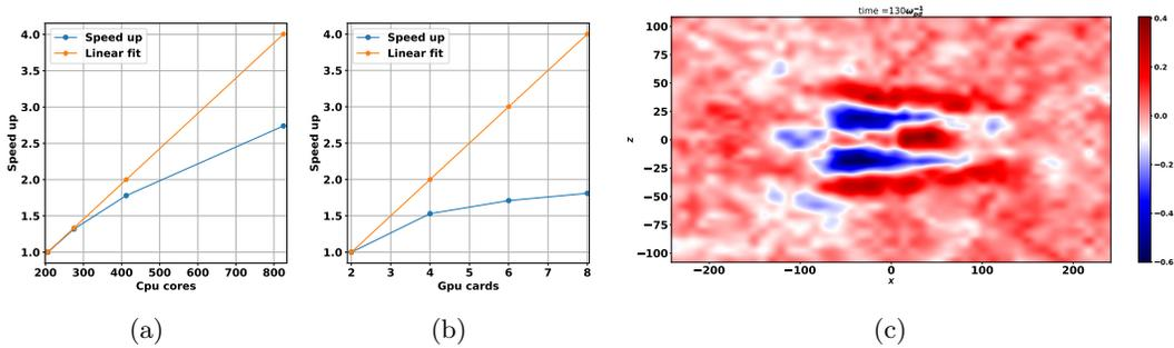
Figure 1: (a) Speed up diagram of the MPI version. (b) Speed up diagram of the multi-GPU version. (c) Spot structure in fluid  $V_x$  velocity field.
