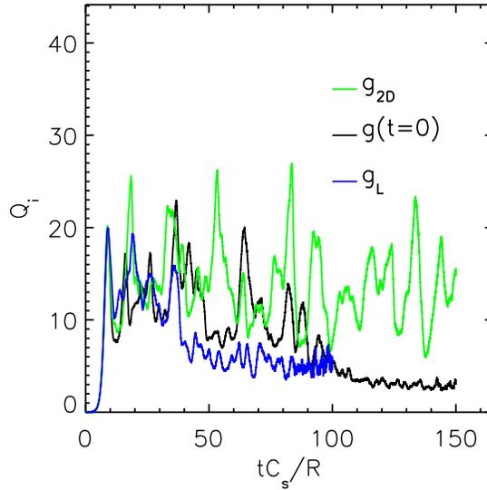
Figure 1: Ion heat flux vs time for three schemes of evaluating the marker distribution: (a) assume the marker distribution is a constant along the trajectory, evaluated during loading (black); (b) the marker distribution is assumed equal to the initially loaded distribution (blue); (c) use the numerical 2-D distribution (green). Only the simulation using the numerical marker distribution maintains a steady state turbulence and transport.
