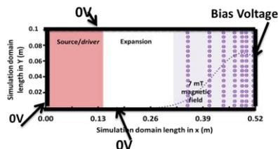
**Figure 1. Simulation domain used in 2D-3V PIC-MCC simulations.**
