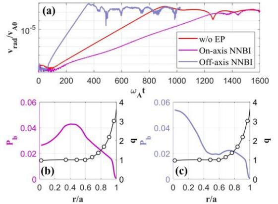
Fig. 1: (a) Comparison of the time evolution of the  $n/m=1/1$  internal kink mode between the MHD, on-axis, and off-axis cases. The bulk plasma pressure profiles of the on-axis and off-axis NNBI cases are shown in panels (b) and (c), respectively.
