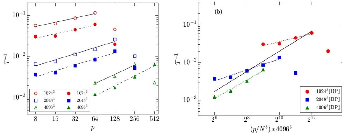
**Figure 1.** Strong (left) and weak scaling (right) of our GPU-FFT. The strong scaling exponent for  $1024^3$ ,  $2048^3$  and  $4096^3$  is 0.34, 0.48 and 0.71 respectively. While weak scaling exponent is 0.9. For all the figures we employ filled symbols for double precision (DP) and unfilled symbols for single precision (SP). Figure from Verma et al. [1].
