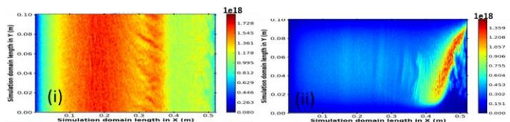
**Figure 2. Snapshots of plasma density (m-3) at 24  $\mu$ s using 2D-3V PIC-MCC model with 7 mT and 20 V bias voltage. (i) without wall and (ii) with wall.**
